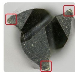
Edge wear after 7 m in CoCr alloy
