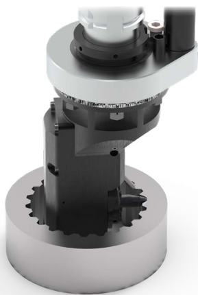
Milling of tooth hub profiles with angle head and carbide tooth form cutter
