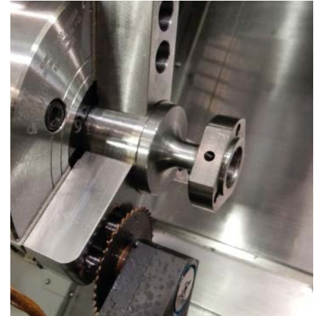
Turn Cut Milling: aluminium Vc = 800 m/min feed = 7m / min
