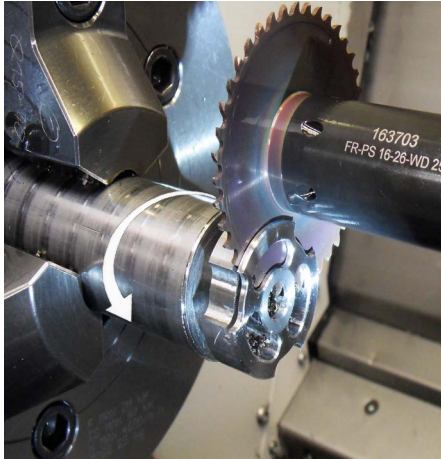
Cutting of VA structured components Vc = 160 m/min Fz = 0,1 mm
